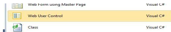
F-37: Add a new item called: “contactForm” by selected the “Web User Control”
